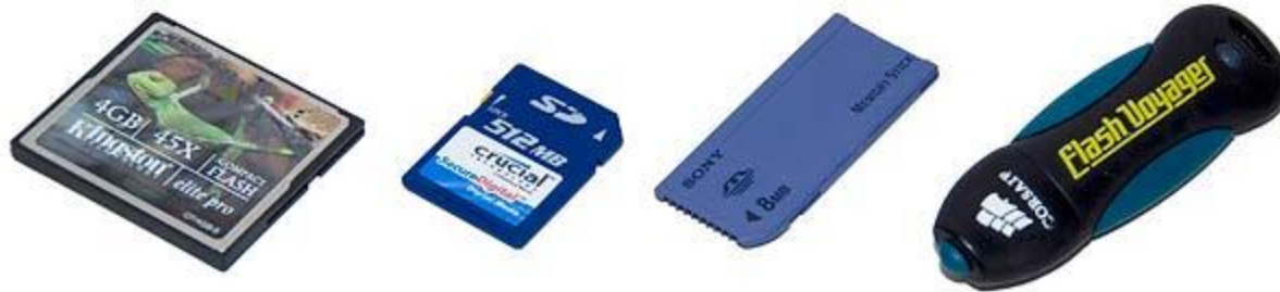
Compact flash (CF) & secure digital (SD) cards, a Sony memory stick, and a USB memory key.
